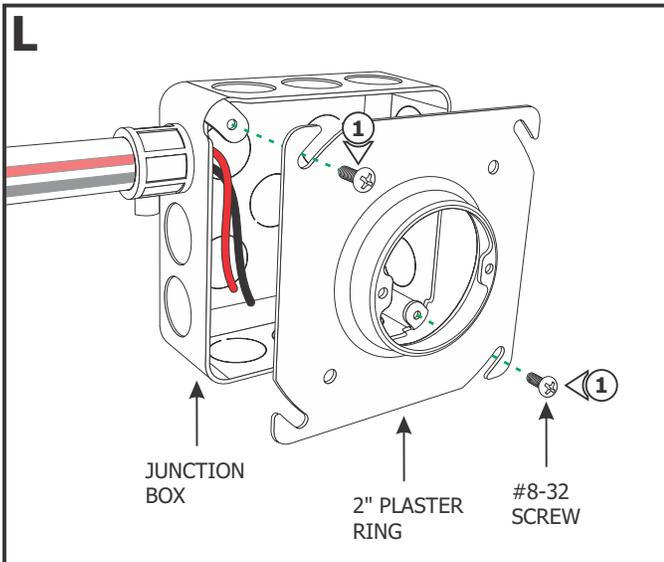
**NOTE:** Junction box must be mounted to allow clearance of 1/2" between the face of the junction box and the drywall surface.
