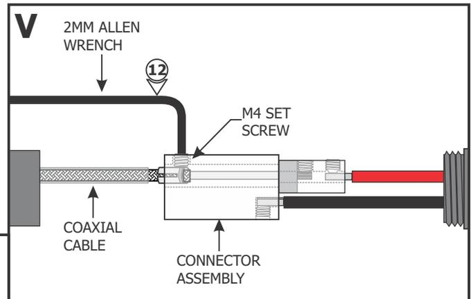
**12:** Use the provided 2mm Allen wrench to securely tighten the M4 set screw until it squeezes the wire ferrule tightly to the coaxial cable.
