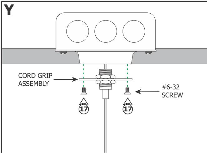
**17:** Mount the cord grip assembly to the 2" plaster ring using two #6-32 screws.
