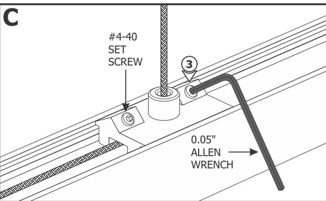
**3:** Place the sliding post back onto the channel and secure it by tightening the two #4-40 set screws with the 0.05" Allen wrench.
