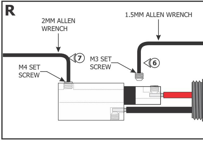
**6:** Using the provided 1.5mm Allen wrench, remove the M3 set screw from the coaxial connector assembly.
