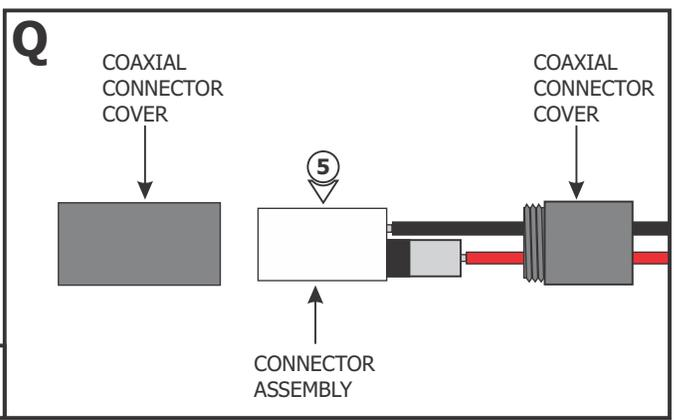
**5:** Unscrew the coaxial connector covers and remove from the connector assembly.
