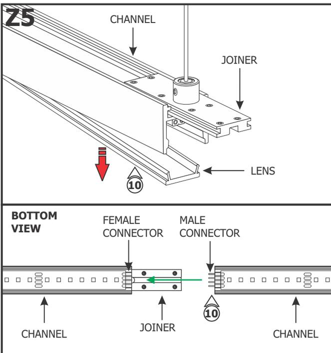
**10:** Lift a section of the lens at the end of the channels where the connectors are visible. Slide the channel over the joiner and ensure the male & female connectors mate properly.
