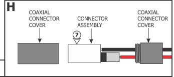
**7:** Unscrew the coaxial connector covers and remove from the connector assembly.
