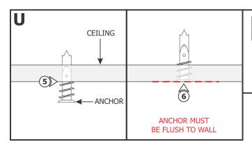
$\underline{\textbf{NOTE:}}$  Steps 5 and 6 are for drywall mounting. Omit these steps if mounting to a wood surface directly.
