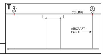
**4:** Lift the other end of the aircraft cables against the ceiling to mark the location of the standoffs.
