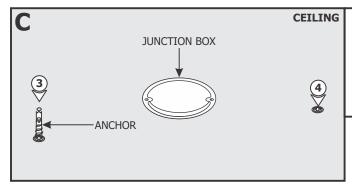
**3:** Align the mounting plate holes with the junction box. Mark one point on each side of the junction box onto the ceiling.
