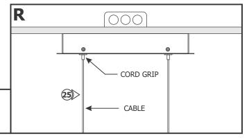
**25:** To make any adjustments to the fixture height, push the cord grips to slide the fixture up and down until the desired height is achieved. Release the cord grips to lock the cables in place.
