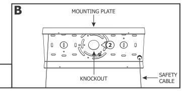
**2:** Select the appropriate knockout on the mounting plate and remove it using a flathead screwdriver or other appropriate tool.
