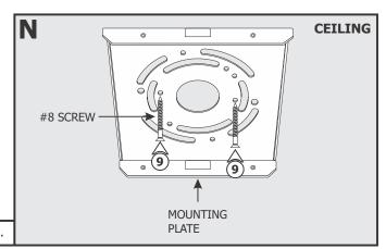
9: Secure the mounting plate to the ceiling using the #8 screws.
