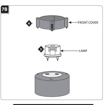
Use ONLY 18 WATT proprietary Element Lighting LED lamp.
