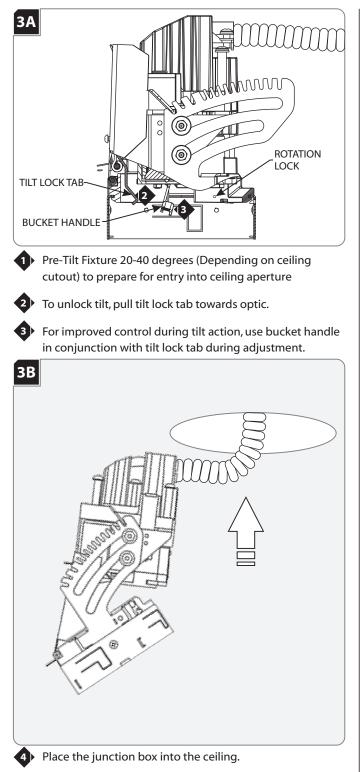
Slide the housing into the hole in the ceiling.
