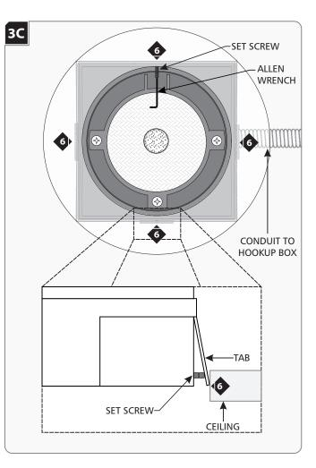
Secure the housing by screwing in the four set screws until they are flush with the inner wall of the housing. Alternate screws before tightening all the way to ensure housing remains centered in the ceiling cutout.
