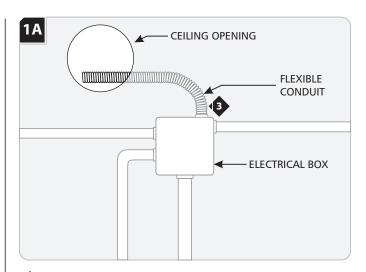
Attach flexible conduit (not included) to an electrical box and feed the conduit out of the hole.
