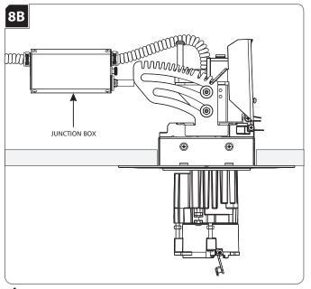
4 Pull the heatsink, module and driver through the aperture.
