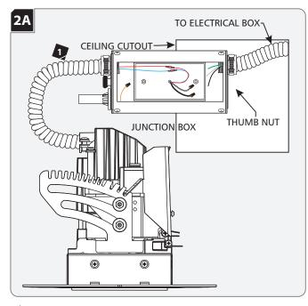
Loosen the thumbnut and remove the cover from the junction box.
