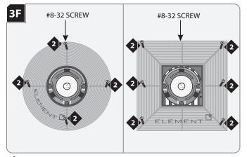
2 Secure the plaster ring in place by screwing the four provided flat head #8-32 screws into the four previously placed drywall anchors.
