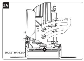
For high position, push up on the center of the LED optic.
