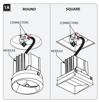
Connect the wall wash module to the fixture using the connectors.
