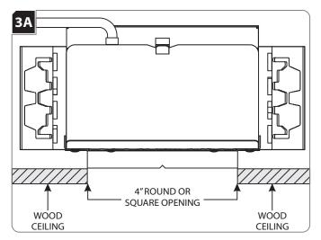
Use a 4" hole saw or mill a 4" square opening in the wood.
