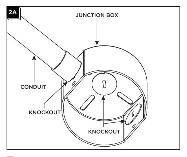
Secure the custom junction box to conduit using one of the three knockouts.
