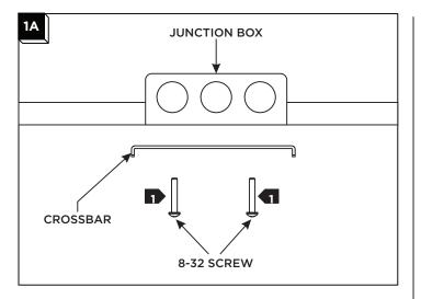
Mount the crossbar to the junction box with the provided #8-32 screws.
