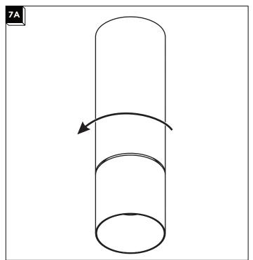
For the adjustable and wall wash fixture: the cylinder can rotate 358° to assist with aiming at the wall.
