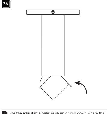
For the adjustable only: push up or pull down where the label is located to tilt the lower cylinder to the desired angle (0°-45°)
