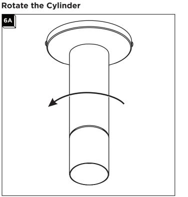
**1** For adjustable and wall wash fixtures: the cylinder can rotate 358° to assist with aiming at the wall.
