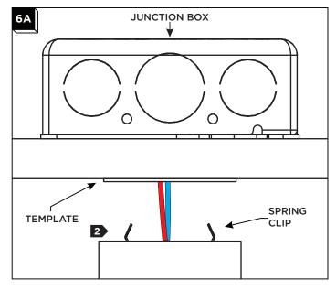
1 Neatly place all wires and wire nut connections inside the junction box.
