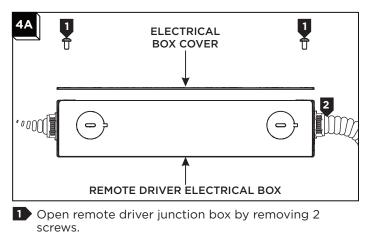
2 Connect conduit or Romex to junction box with the proper fittings
