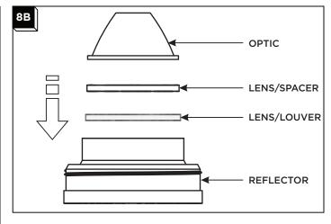
3 In the accessory reflector place the first lens or louver.
