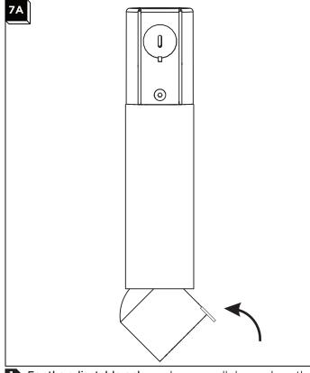
1 For the adjustable only: push up or pull down where the label is located to tilt the lower cylinder to the desired angle (o°-45°)
