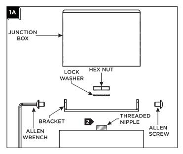
Separate the junction box from the bracket, use the provided Allen wrench to remove the two Allen screws securing the bracket to the junction box. Save the screws for reassembly later.
