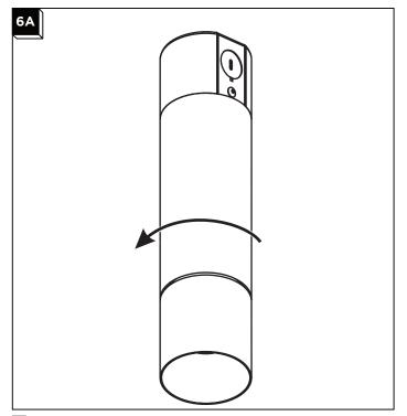
For the adjustable and wall wash fixtures: the cylinder can rotate 358° to assist with aiming at the wall.
