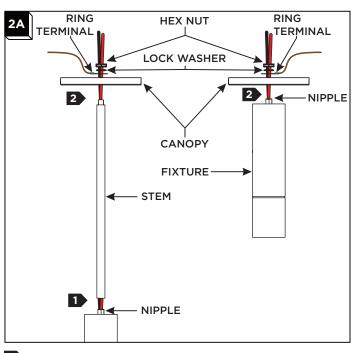
For Optional Stem: If the optional stem was ordered feed the wiring through the stem first and screw the stem to the top of the fixture.
