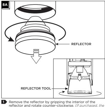
reflector and rotate counter-clockwise. (If purchased, the reflector tool can be used to grip the reflector.)
