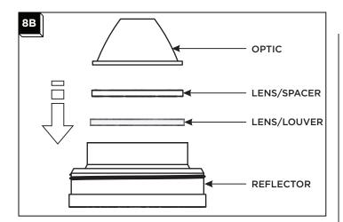
3 In the accessory reflector place the first lens or louver.
