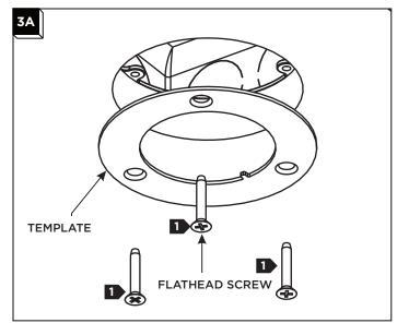
Use the three flathead screws to secure the template to the previously installed J-box plate.
