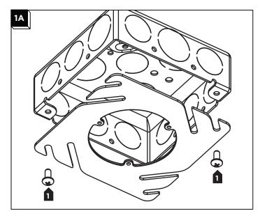
Prior to installing the drywall, attach the support plate to the junction box with the provided screws.
