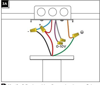
Use the following wiring diagram to wire your fixture.
