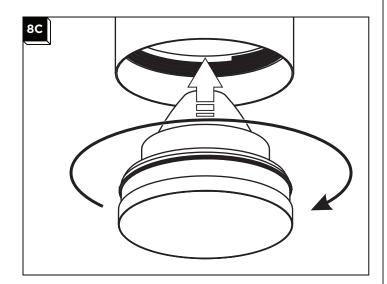
6 Install the reflector by inserting it into the bottom of the Cylinder and screw it in as far as it will go.
