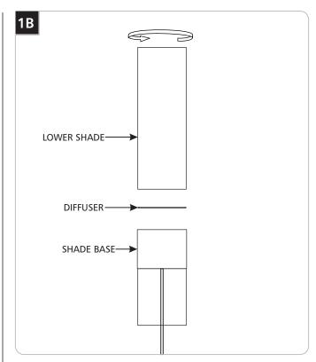
Rotate the fixture upside down, place the diffuser into the shade base, and completely screw the (longer) lower shade into the base.
