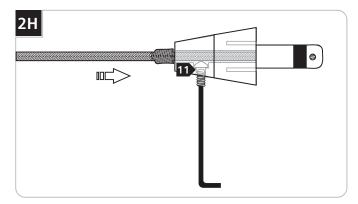
11 Firmly tighten the set screw on the conical connector.
