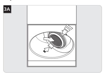
**WARNING:** Always squeeze the two tabs when adjusting the LED housing. Failure to do so will damage the finish.
