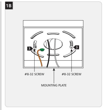
Secure the mounting plate to the electrical box with the two provided #8-32 screws.
