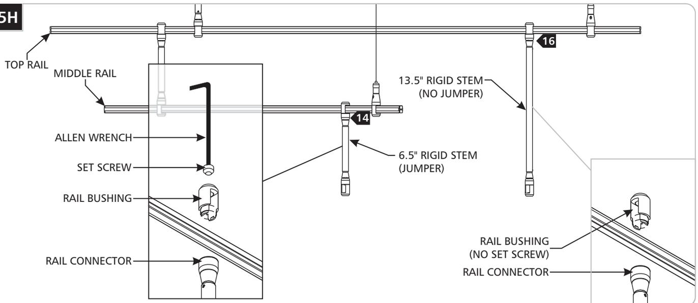
**CAUTION: Do not mix parts on the rigid stems. 6.5" stems are conductive and 13.5" stems are non-conductive.**
