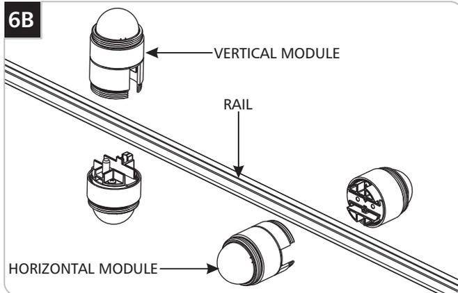
**CAUTION:** Make sure to disconnect the power to the fixture when installing the modules. Failure to do so may result in damage to the fixture and/or injury.
