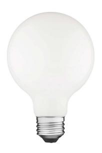
FINISH Frosted LAMP G25/Medium (E26)/120V LED WATTAGE 5W DIMMER Incandescent DIMENSIONS 3.2"W x 4.7"H Technical Information LUMINOUS FLUX 500 lumens LUMENS/WATT 100.00 COLOR TEMPERATURE 1800K-3200K Warm Dim COLOR RENDERING 80 CRI
