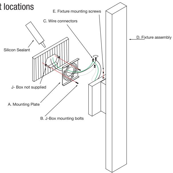
**Installing the fixture *please ensure the electrical breaker is switched off before commencing***
