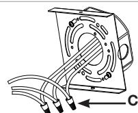
3 Attach the Fixture assembly (D) to the Fixture mounting plate (A) and with the supplied Fixture mounting screws (E) and secure top and bottom. Caulk the mounting plate with a suitable silicon sealant to prevent moisture entering the fixture.
