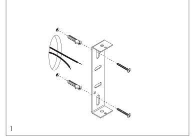
Disconnect the power by turning off the circuit breaker, or by removing the fuse in the fuse box before assembling and mounting the canopy. Fix the mounting plate to the ceiling with dowels and screws.
