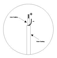
coax cable requires ping of outer and r coatings to access tive and negative rection wires
