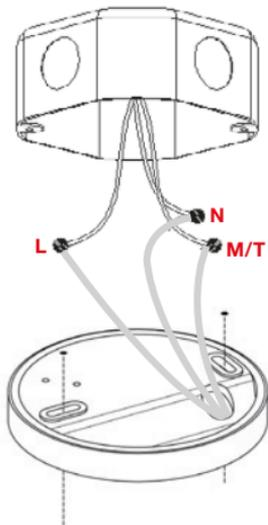
**EN** Make sure that the wires do not spill out excessively as shown in the diagram.
