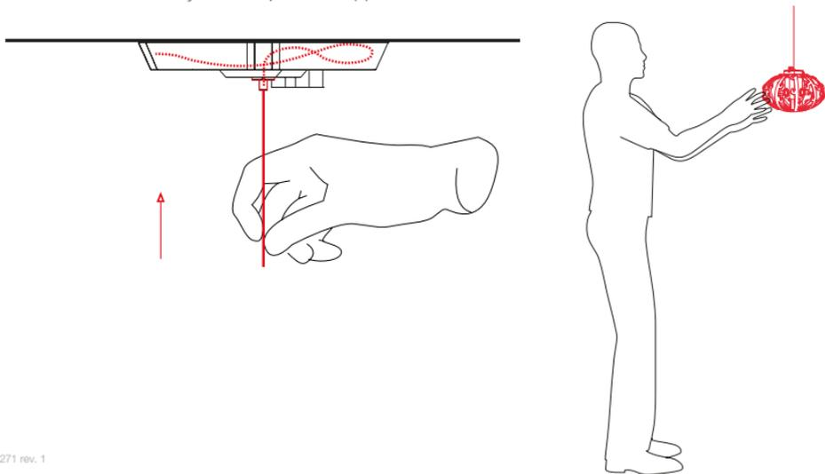
**EN** If the metallic wire has been pushed up too far it can be recovered by releasing the stop exerting a pressure with a finger on the small piston shown in red in the picture, and then insert the light bulbs. Insert the bulb into the tool provided (9). Mount the bulb in the socket and press the plunger until the bulb releases.
