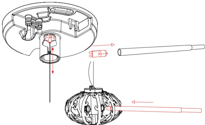
**EN** Attach the flowers (6) to the frame lodging them in their positions following a spiral pattern starting from the central flower. For the multicolour version, the positioning of the arrangement of the shades of the flowers can be customised. Adjust the lamp to the desired height. The height of the lamp on the base can be adjusted using the base piston as previously described.
