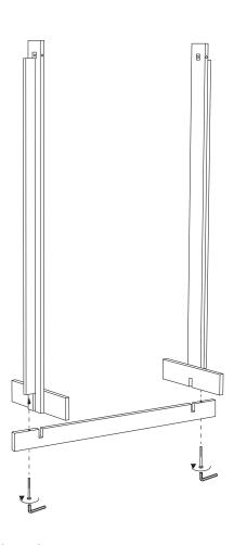
Place the two side panels on the bottom bar. Screw in two screws from the bottom.
