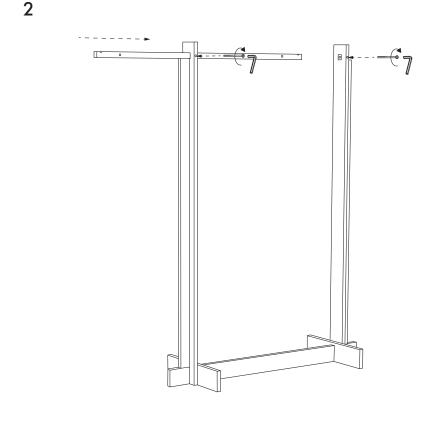
Push the top pin through the holes in the side panels. (The notch in the top bar must face up) Screw in two screws in each side panel.
