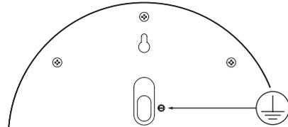
3 Make the appropriate electrical connections.
