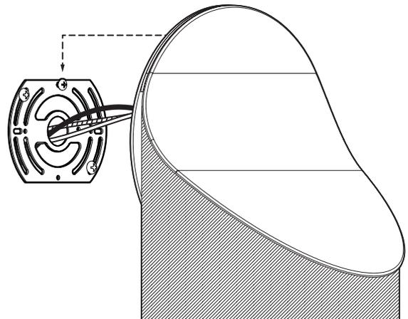
4 Once connected, mount the lamp on the wall by sliding the head of the screw in the aperture situated above the junction box.
