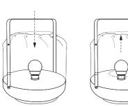
Install/change the bulb in the lampholder.
