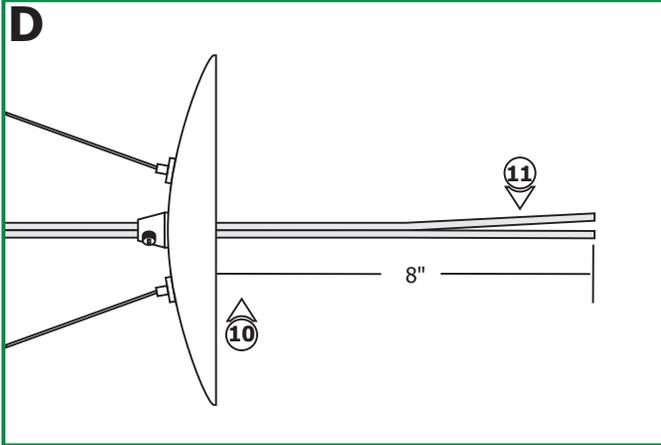
**10:** Leave 8" of the clear cord exposed behind the canopy for power connection. Trim off the excess clear cord.
