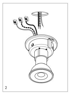
Fix the lamp cables to the current electricity with the connectors.
