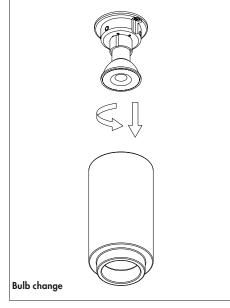
Disconnect the power by turning off the circuit breaker, or by removing the fuse in the fuse box before. Pull off the barro negro from thechnic.
