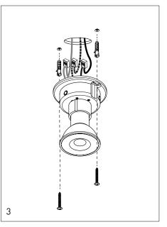
Fix the mounting to the ceiling with the dowels and screws.
