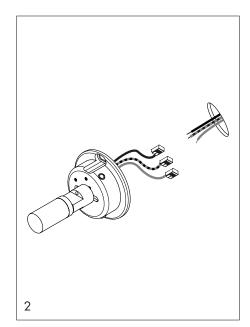
Fix the lamp cables to the current electricity with the connectors
