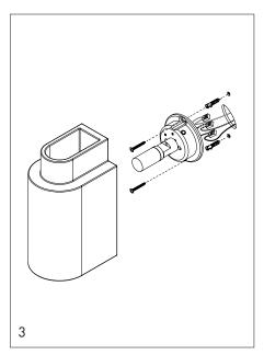
Fix the mounting to the wall with the dowels and
