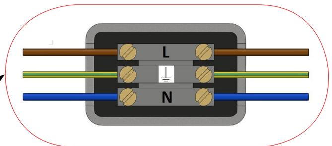
**7.** Connect the mirror wiring in an IP44 approved connector box (not included) which can be inserted into the wall anywhere behind the cabinet mirror.
