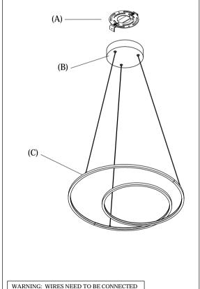
TO DRIVER FOUND IN CANOPY AND SHOULD NOT CONNECT DIRECTLY TO POWER SOURCE
