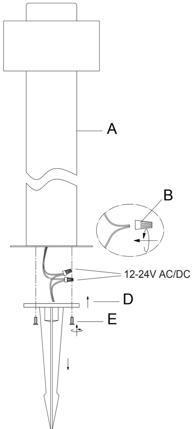
For outdoor use,caulk around fixture with silicone sealant to prevent water intrusion. leave a gap at the bottom allow moisture to escape.
