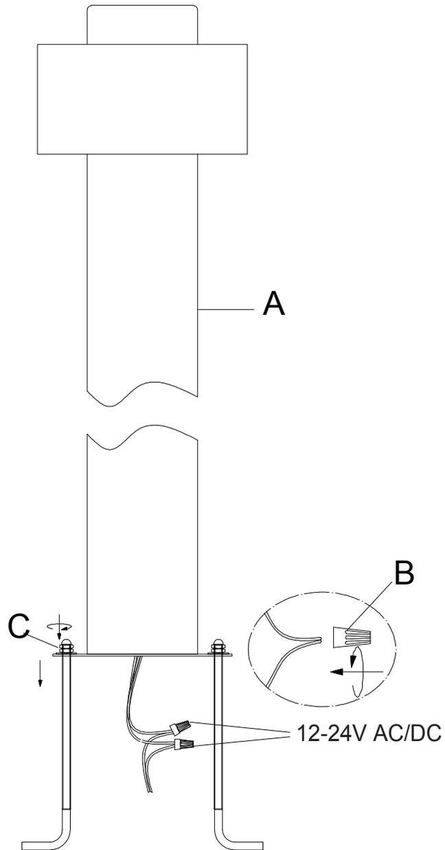
For outdoor use,caulk around fixture with silicone sealant to prevent water intrusion. leave a gap at the bottom allow moisture to escape.
