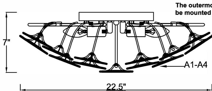
The outermost glass for A4 should be mounted with an incline.
