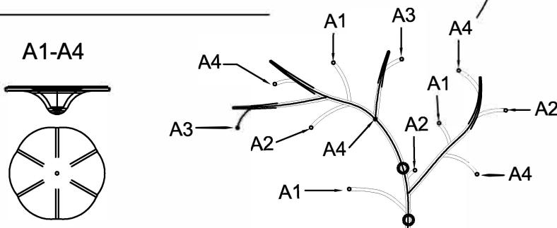
There are three sets of branches on the frame. The branches are labelled with the stickers A1, A2, A3, or A4 which indicates where the glass is supposed to be attached. Please follow the guidance of these stickers to install the glass on all of the branches.
