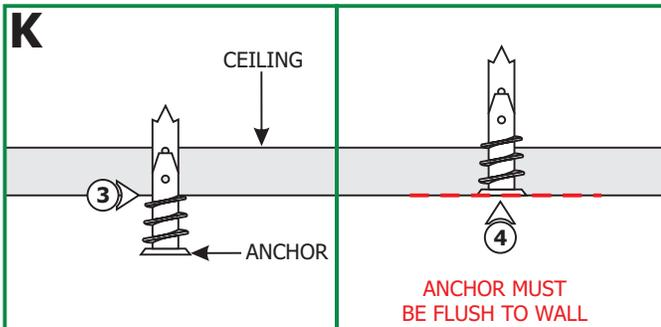
**NOTE:** Steps 3 and 4 are for drywall mounting. Omit these steps if mounting the clips to a wood surface directly.
