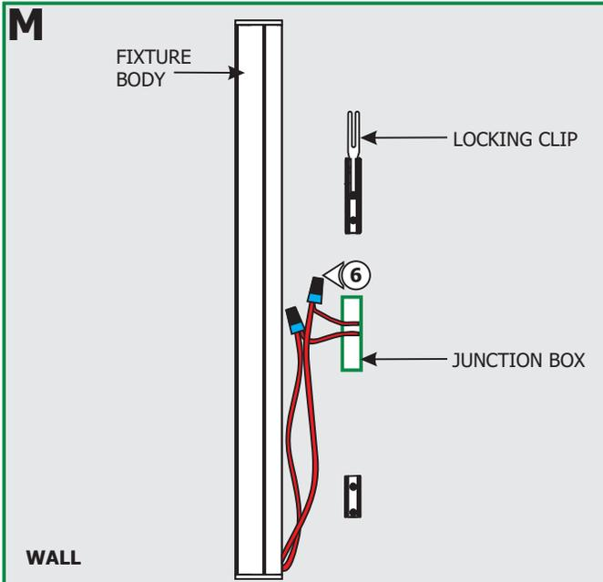
**6:** Connect each power supply wire to a fixture body wire with a wire nut.
