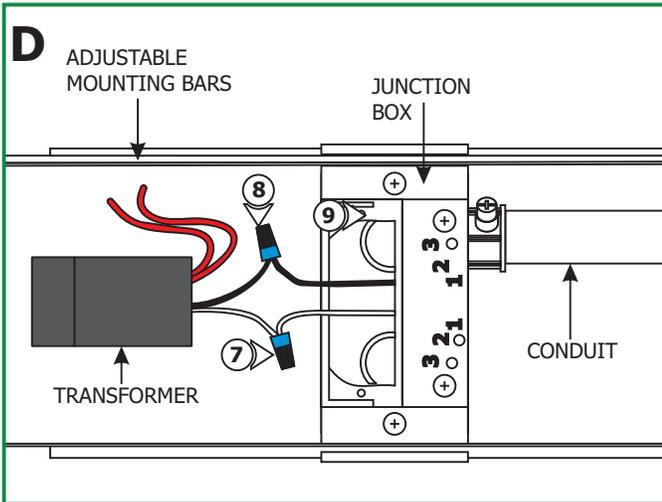
**NOTE:** If necessary junction box opening can be adjusted to two positions: Position 2 at 0.95" (recommended for this installation), or Position 3 at 1.05". Simply loosen screws and tighten to the corresponding position labeled on junction box. **POSITION ONE SHOULD NOT BE USED FOR THIS INSTALLATION** as it will not allow access to the LED transformer after installation.
