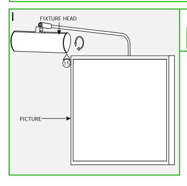
15: Rotate the fixture head to properly wash the picture with light.
