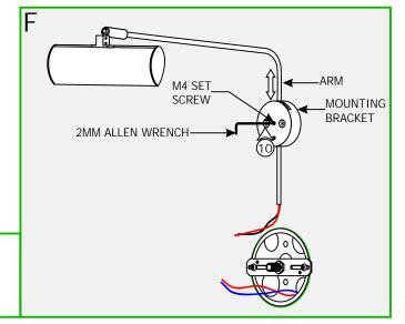
10: To adjust the Cody2 height, loosen the two M4 set screw on the mounting bracket with the provided 2mm Allen wrench. Adjust the Cody2 by sliding it up or down. When the desired height is achieved tighten the two M4 set screws with the 2mm Allen wrench.
