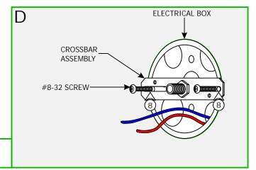
8: Mount the crossbar assembly to the electrical box holes with the provided #8-32 screws.
