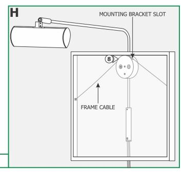
**8:** Hang the frame cable in the mounting bracket slot.
