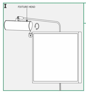
**9:** Rotate the fixture head to properly wash the picture with light.
