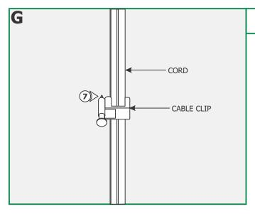
**7:** Use the provided cable clips to secure the cord to the wall, or use a cable cover (not provided)
