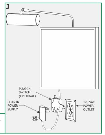
**10:** Use the plug-in switch (optional) in line with the plug-in power supply and outlet to turn the fixture on and off. DO NOT install any other switch to the cord. This may result in damage to the LEDs.
