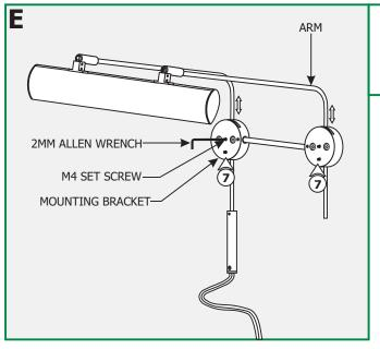
7: To adjust the height, loosen the four M4 set screw on the mounting brackets with the provided 2mm Allen wrench. Adjust the Cody to the desired height by sliding it up or down. Tighten the four M4 set screws with the 2mm Allen wrench.
