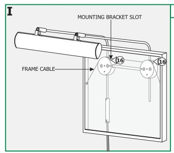
**16:** Hang the frame cable into the two mounting bracket slots.
