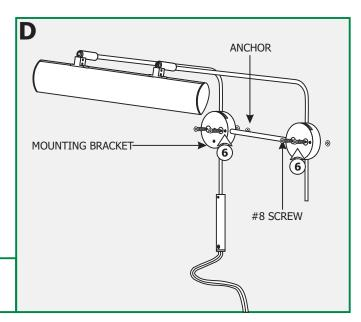
**6:** Line up the mounting bracket holes with the anchors and secure the fixture to the anchors with the four #8 screws provided.
