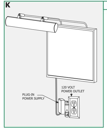
18: Plug the power supply into the 120 volt power outlet.
