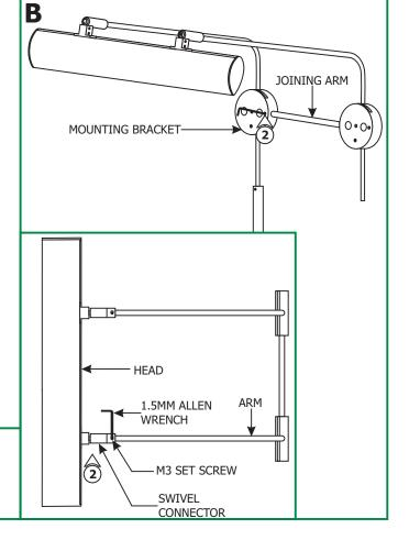
2: Insert the loose arm assembly (provided in the box) into the other swivel connector and insert the joining arm into the mounting bracket of the first arm. Tighten the M3 set screw on the swivel connector and mounting bracket with the 1.5mm Allen wrench.
