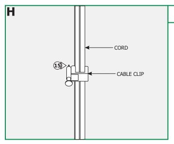
**15:** Use the provided cable clips to secure the cord to the wall, or use a cable cover (not provided)
