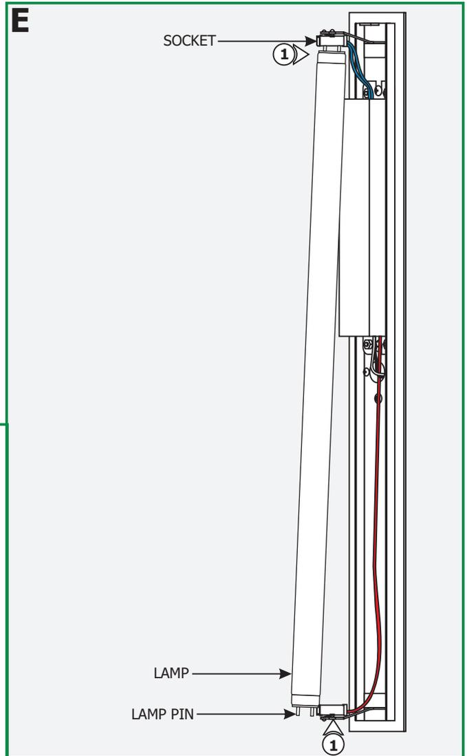
**CAUTION:** To reduce risk of a burn or electrical shock during lamping, disconnect the power to the fixture.
