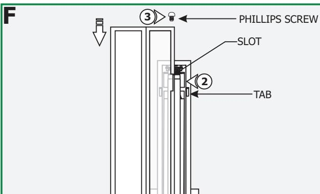
**2:** Align the glass shade slots with the fixture tabs. Push the glass shade onto the fixture and slide it to lock in place.
