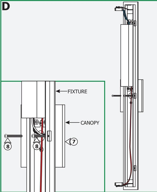
**7:** Place all wires and wire nut connections properly inside the electrical box.
