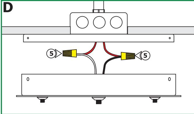
**4:** Make sure that the mounting plate is grounded in accordance with local electrical codes.
