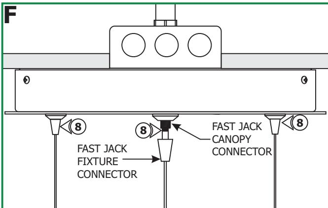
**CAUTION: Risk of Fire:** The total load of the Fast Jack canopy ports should not exceed the remote transformer rated capacity.
