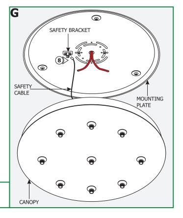
**8:** Insert one end of the safety cable into the safety bracket of mounting plate and the other end into the canopy safety bracket.
