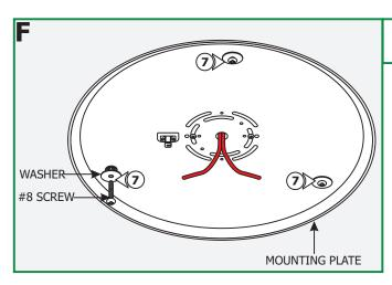
**7:** Secure the mounting plate to the anchors with the provided #8 screws and washers.
