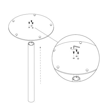
Mount the table base on the column with 3 (A) counter sunk screws.
