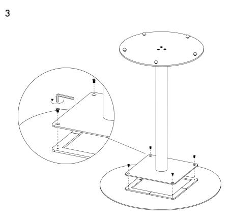
Lay the table top on a blanket and mount the table leg with 4 (B) counter sunk screws.
