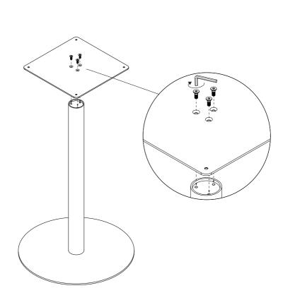
Mount the Connection plate on the column with 3 (A) counter sunk screws.
