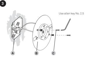
Fix the electrical back plate (B) to the junction box (A) with the screws (C).
