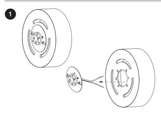
Remove the electrical back plate by detaching it from the shade.
