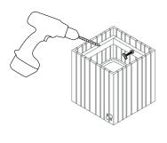
5. Make sure that the product is well fixed to the wall. The screw with the raw-plug needs to carry the weight of min. 8kg.
