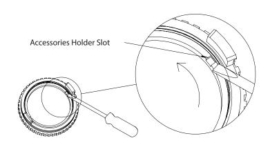
4. Fixture accommodates one lens and one glare control accessory. Refer to spec sheet for list of compatible accessories. Install accessories between the front cap and accessory holder. Tighten accessory holder after accessories are installed. (Fig.7)
