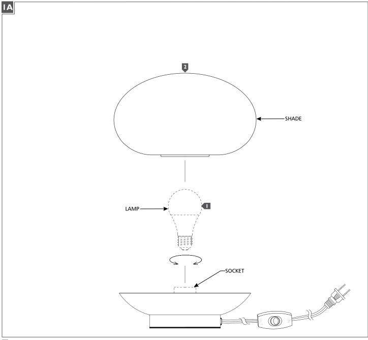
Screw the lamp into the socket. Refer to the label on the lamp socket for Max Wattage Information.
