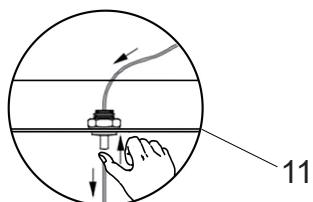
**Note:** Press the wire restraint to adjust the desired length of cable.
