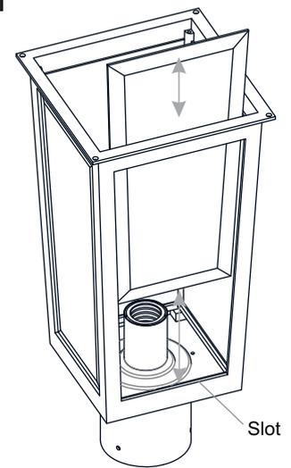
Reverse the above steps to reinstall the glass holder and the cage.
