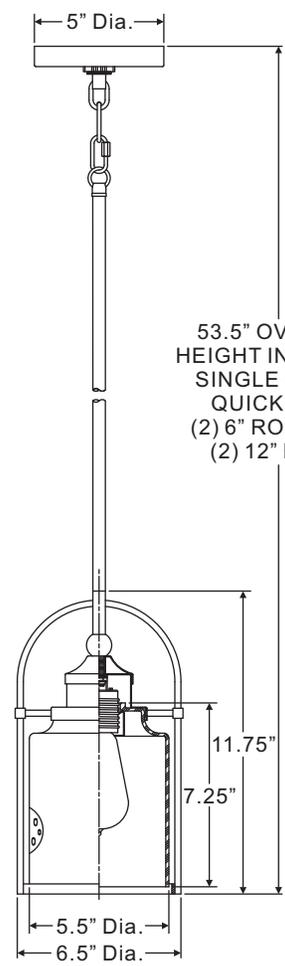
53.5" OVERALL HEIGHT INCLUDES SINGLE CHAIN, QUICK LINK, (2) 6" RODS AND (2) 12" RODS
