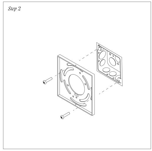
Mount the backplate to the junction box using a phillips head screwdriver to tighten two mounting screws. Make sure the wires from the junction box are still accessible.
