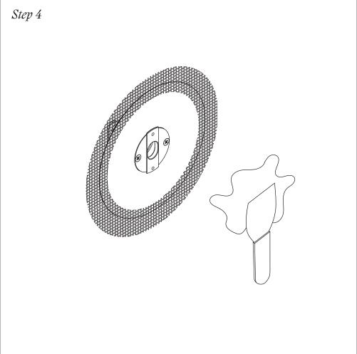
Mount the Mud-ring to the junction box using a phillips head screwdriver to tighten two mounting screws. Make sure the wires from the junction box are still accessible.
