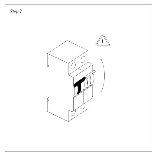
Turn the power back on at the main fuse box or circuit panel you disabled before installation. Turn on the light :)
