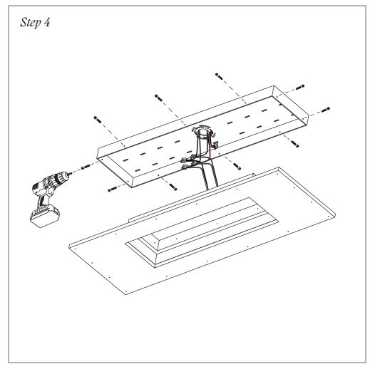
Align the holes of the backplate with the holes of the canopy cover. Secure the canopy cover in place using the canopy screws, a drill and the 5/32" Hex drill bit provided.
