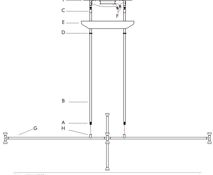
04. Gently lower down the wooden canopy (A) through the stems (B) so it can rest. Be careful not to scratch the finish.
