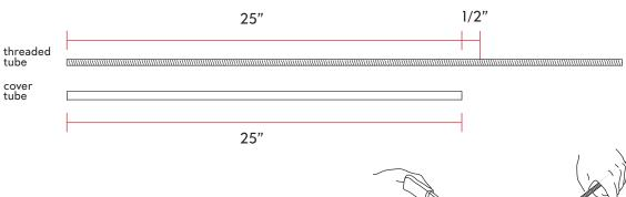
4. Hold down the all thread with a hand or a clamp, use a hacksaw or electrical tool to cut the all thread tube. Recommended to clean all thread tube after cutting to remove any metal chippings.
