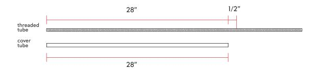
4. Hold down the all thread with a hand or a clamp, use a hacksaw or electrical tool to cut the all thread tube. Recommended to clean all thread tube after cutting to remove any metal chippings.
