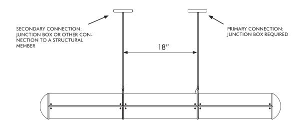
Standard 5 unit configuration with hanging points separated by 3 units:
