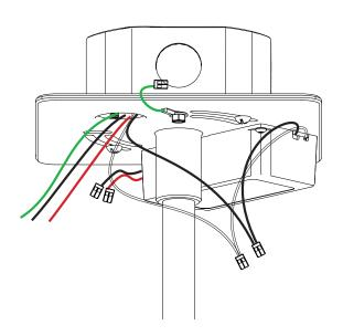
7. Make the electrical connection between the J-box and fixture.
