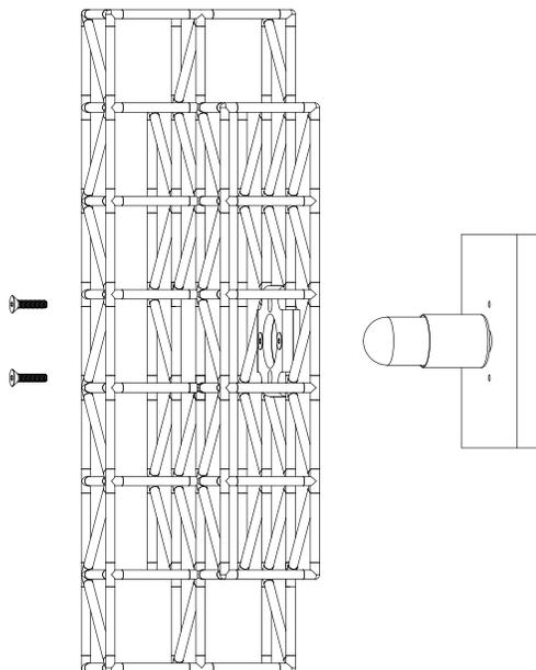
6. Use the provided T-handle driver to reach through the cage and tighten the allen screws.
