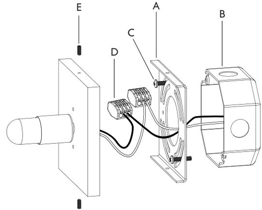
5. Lift the cage body and fit the hole over the socket assembly. Attach the 8-32 Allen Screws through the top and bottom holes on the face of the backplate body.
