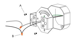
4. Tuck wires (and transformer when applicable) into canopy and tighten back on to crossbar with two brass screws.
