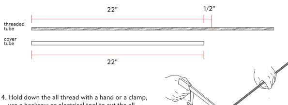
4. Hold down the all thread with a hand or a clamp, use a hacksaw or electrical tool to cut the all thread tube. Recommended to clean all thread tube after cutting to remove any metal chippings.
