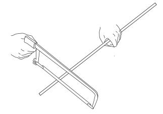
3. Now that the cover tube is cut to 20", measure the all thread tube to be 20 and 1/2" long. And place a mark, with a marker or tape.
