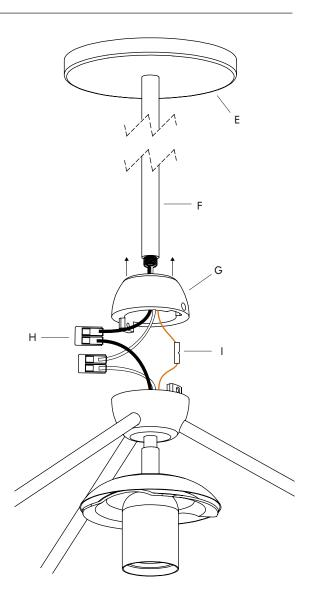
8. Secure the two half hubs together using a hex key and the provided #6-32 socket screws on either side.
